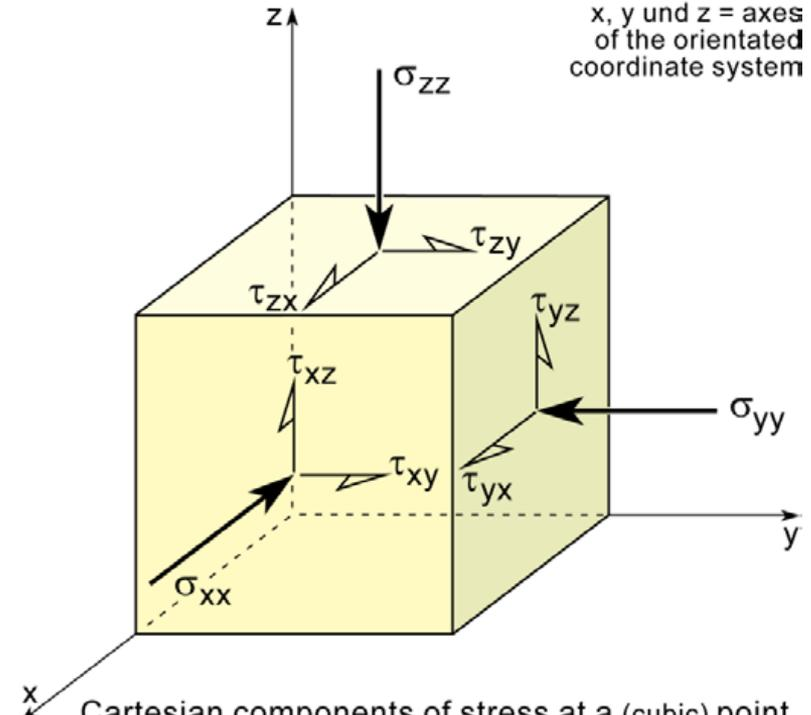
Cartesian components of stress at a (cubic) point resolved into normal- ( $\sigma$ ) and shear- ( $\tau$ ) stress components
