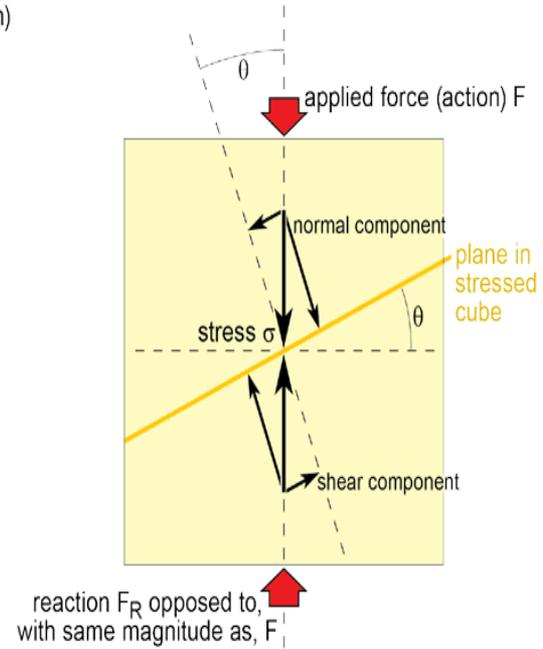
Stress (a pair of equal and opposite vectors) induced at a point of an inclined plane within a body subjected to uniaxial compression
