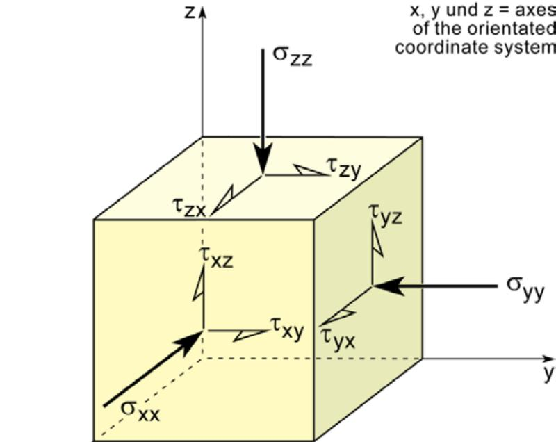
Cartesian components of stress at a (cubic) point resolved into normal- ( $\sigma$ ) and shear- ( $\tau$ ) stress components
