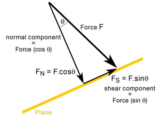
Vectorial decomposition of a force applied to a plane into its normal- and shear components
